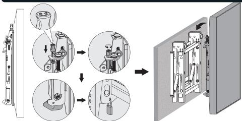
Note: Before hooking the display, make sure the knobs are rotated to the unlock position.
