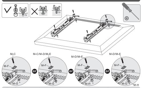
Note: Choose the appropriate screws, washers and spacers (if necessary) according to the type of screen.
