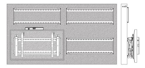
Adjust the display to keep level in vertical and horizontal directions.
