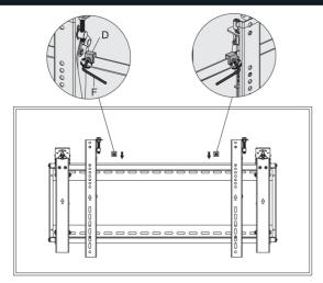
Install the both antiskid blocks as close to the adapter brackets as possible. Tighten screws on the antiskid blocks using an Allen key to prevent display from moving.
