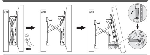
Push the display inward and then release it, the display will be pop-out. Kickstands provide tilt access for easy cables management and maintenance.
